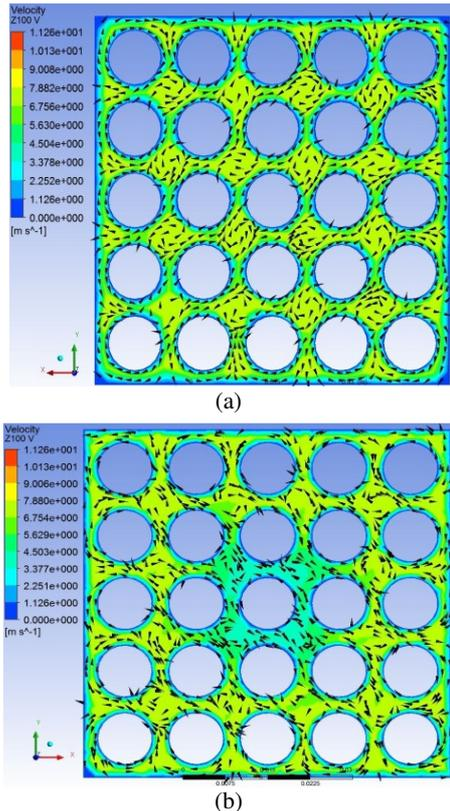
Fig. 4 Velocity vectors and profile at  $z = 100\text{mm}$  downstream the spacer grid without blockage (a) with blockage (b).
