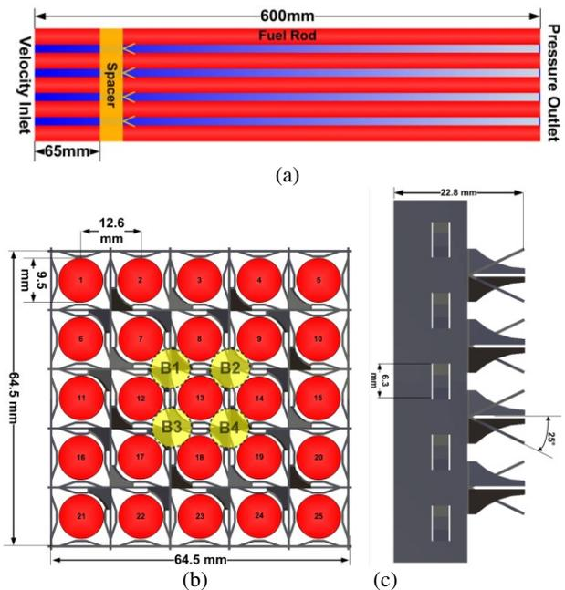
Fig.1 Computational domain (a) with details of the spacer grid (b) and the vanes (c).
