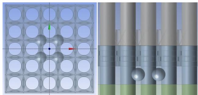
Fig. 2 Location of simulated insulation debris.
