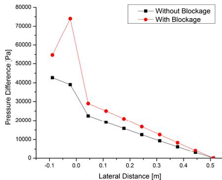
Fig. 5. Pressure distribution at the channel B1.
