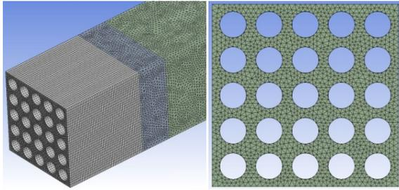
Fig. 3 Meshes in the computational domain (a) and velocity inlet (b).
