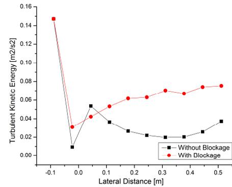
Fig 7. Turbulent kinetic energy profiles at the center of channel B1.
