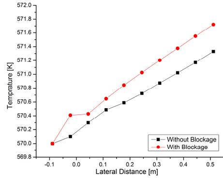
Fig 6. Bulk temperature profiles at the center of channel B1.
